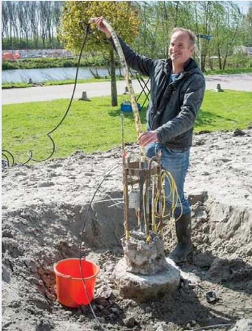
**Figure 5** – The seismic tube is placed in the hole in a pile.
