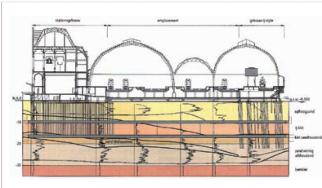
**Figure 2** Geotechnical longitudinal profile.
