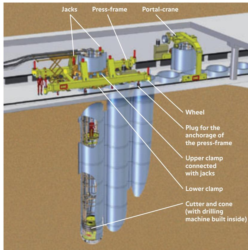
**Figure 3** Detail of the press frame and representation of the production process of the MT-piles.
