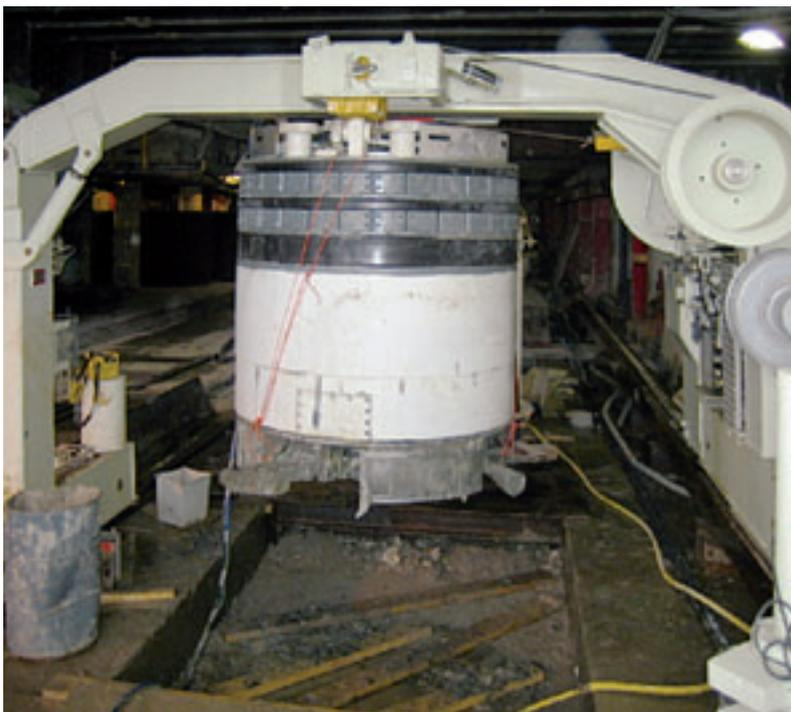
**Photo 1** The drilling machine and the cutter wheel hang in the portal-crane.
