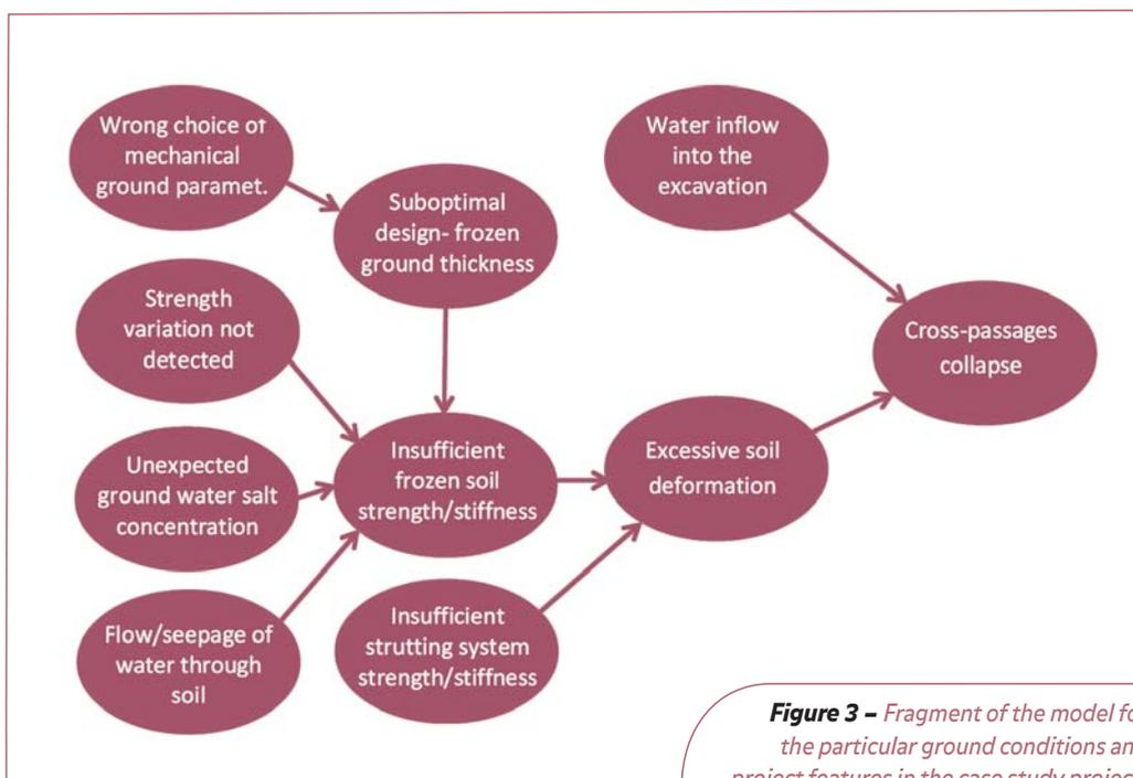
**Figure 3** – Fragment of the model for the particular ground conditions and project features in the case study project.
