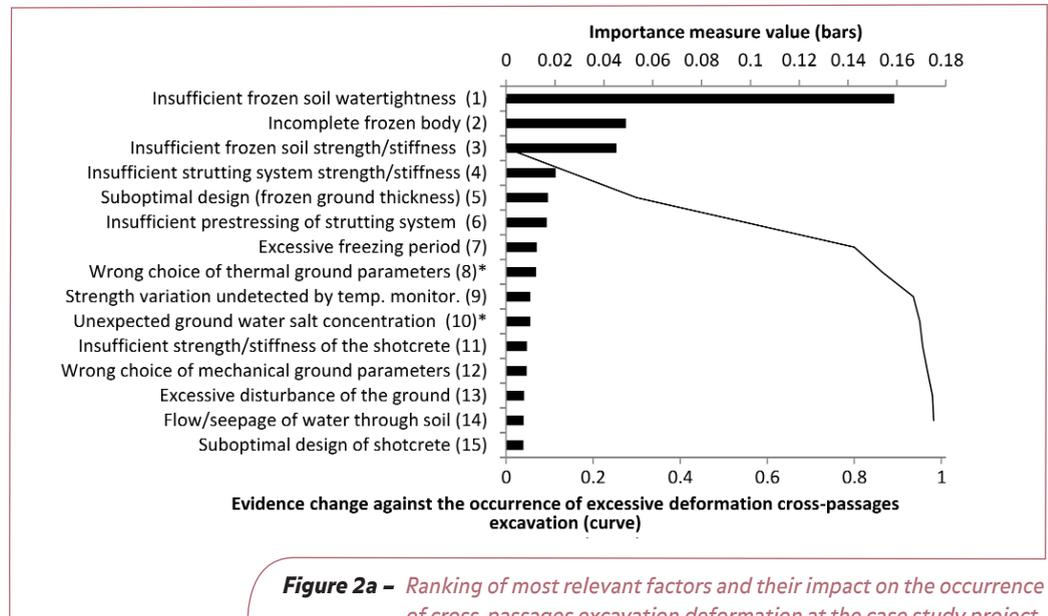
Figure 2a – Ranking of most relevant factors and their impact on the occurrence of cross-passages excavation deformation at the case study project.
