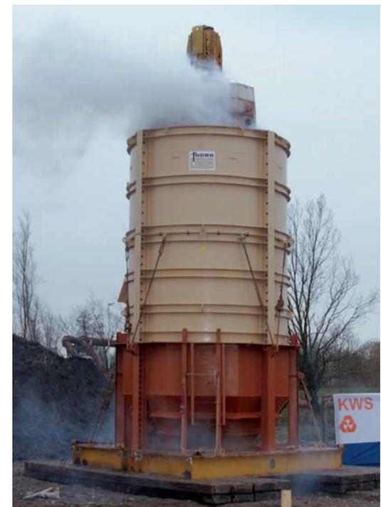
**Figure 4** 16 MN Statnamic load test.
