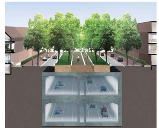
Figure 4 Double stacked tunnel A2 Maastricht. Source: Avenue2.
