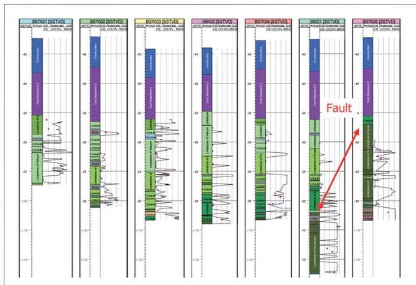
Figure 2 Adjacent boreholes. Blue represents the top soil, purple the gravel layer, the green colours the different members of the Formation of Maastricht and brown the Formation of Gulpen. The black line indicates the pocket penetrometer readings.
