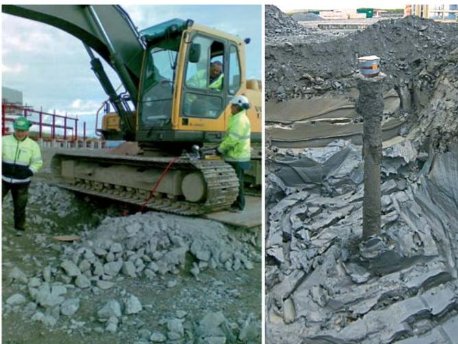
**Figure 2** Test loading and over 4 m exposed HSP pile.
