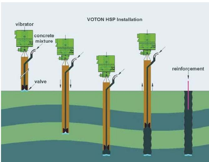
**Figure 3** Schematic view of the installation of HSP piles ([www.voton-hsp.com](http://www.voton-hsp.com)).
