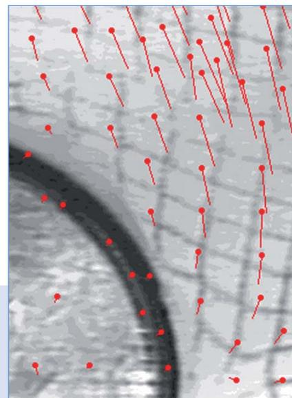
**Figure 3** Movement of consolidating clay around a tunnel. Result of centrifuge test.
