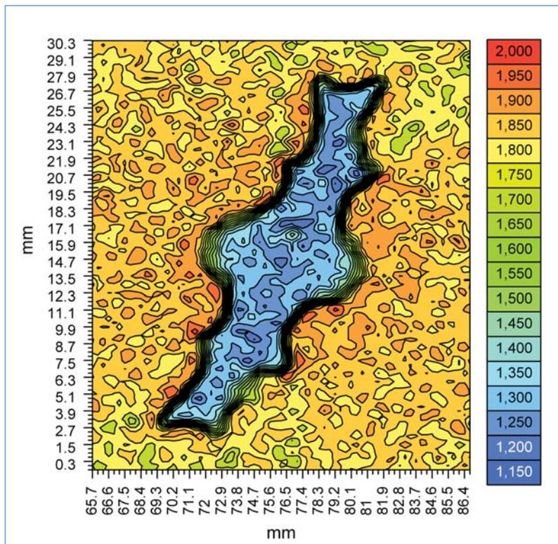
**Figure 2** Density of a fracture in sand with a WCR of 10. The blue is the fracture, the orange-yellow-green the sand.
