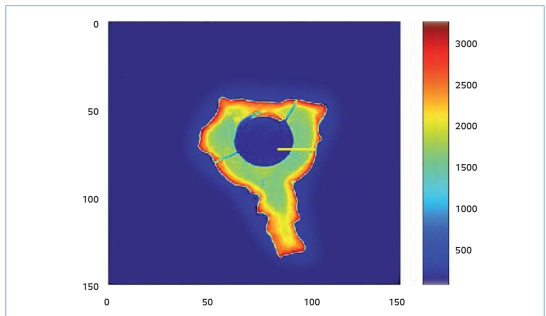
**Figure 1** Attenuation of x-rays over a grout sample with a WCR of 1. The surrounding air is blue. Red is the highest density ( $2100 \text{ kg/m}^3$ ), green the lowest ( $1500 \text{ kg/m}^3$ ).
