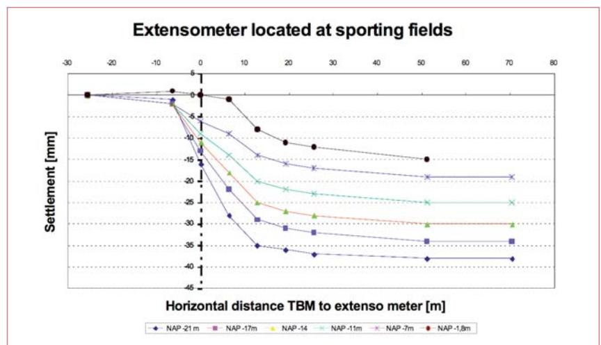
Figure 6 Settlement in time above tunnel
