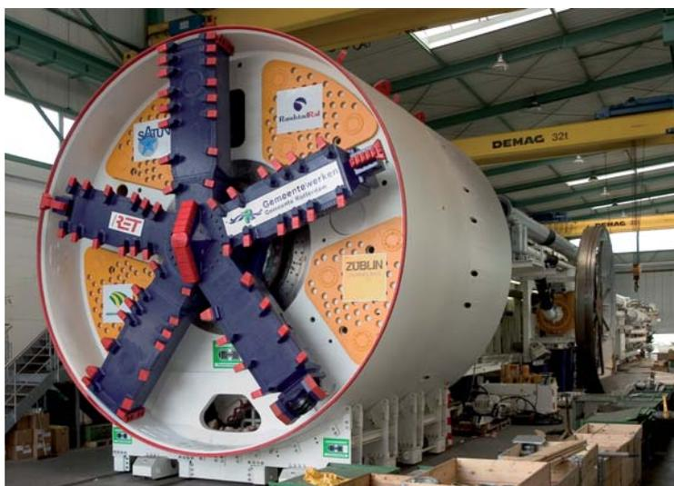
Figure 5 RandstadRail Tunnel Boring Machine (TBM).
