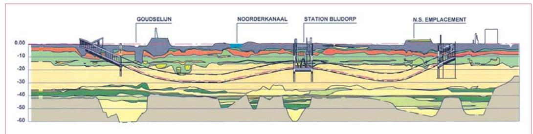
**Figure 3** Vertical alignment of bored tunnels; distance start tunnel – Blijddorp station – Rotterdam CS station ca. 2,0 & 1,2 km.
