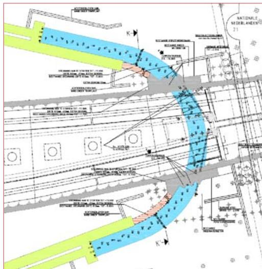
**Figure 9** Plan of designed collar construction around the tunnel at station platform elevation, showing frozen soil area (blue) and supporting diaphragm walls (green).
