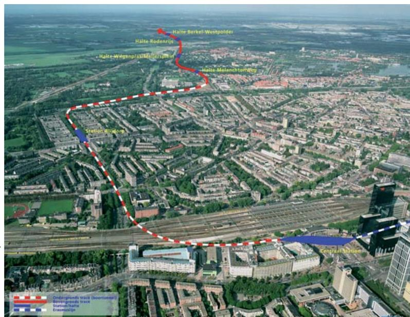
Figure 2 Alignment of RandstadRail in Rotterdam.
