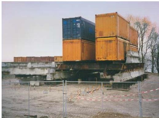
**Figure 10** Test site for the Pile-tunnel interaction test.
